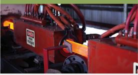
Tejas Tubular is the industry leader in heat treat and has set the benchmark for the heat treatment of coupling stock.
