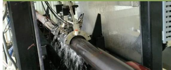
**Tejas Tubular has a custom & automated Full Body Ultrasonic Inspection system to inspect its tubing pup joints.**
