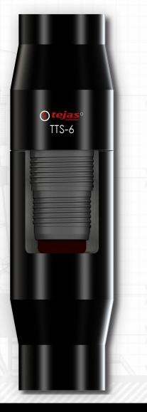
The Tejas Tubular TTS-6 is a industry known thread design connection for use in production tubing and work string applications. The dual step design on upset ends provides trouble-free stabbing and make-up with superior galling resistance. The 100% tensile, 100% internal pressure and 100% collapse efficiency, along with high torque strength, provides a trouble-free connection for any HT/HP application.
